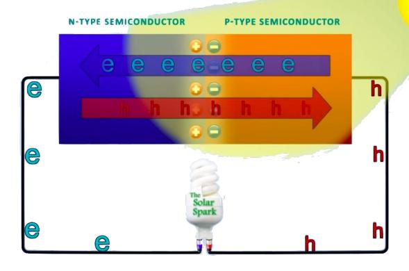
If you were to connect the junction to a circuit, the charges driven around the circuit forms an electric current. This allows us to power things, like light bulbs.
